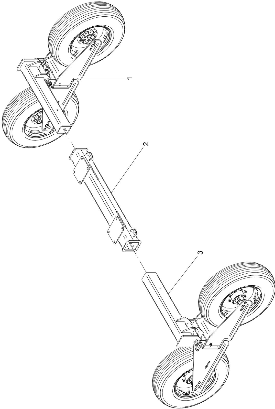
40 - KIT EIXO TANDEM PNEU RIB RA45 10.5/80-18 10 LONAS – 23004800
