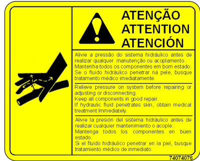
Code: 74074076 - Relieve hydraulic system pressure.
