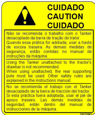
Code: 74121041 - It is not recommended to operate the machine disconnected from the tractor drawbar.
