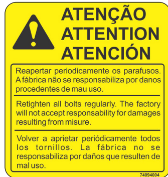
Code: 74094004 - Retighten the bolts periodically.
